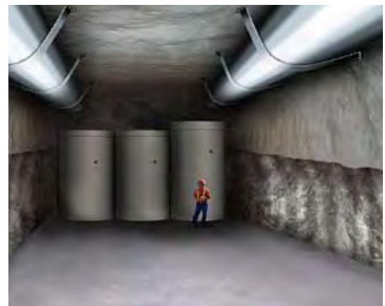
Intermediate level waste emplacement room
